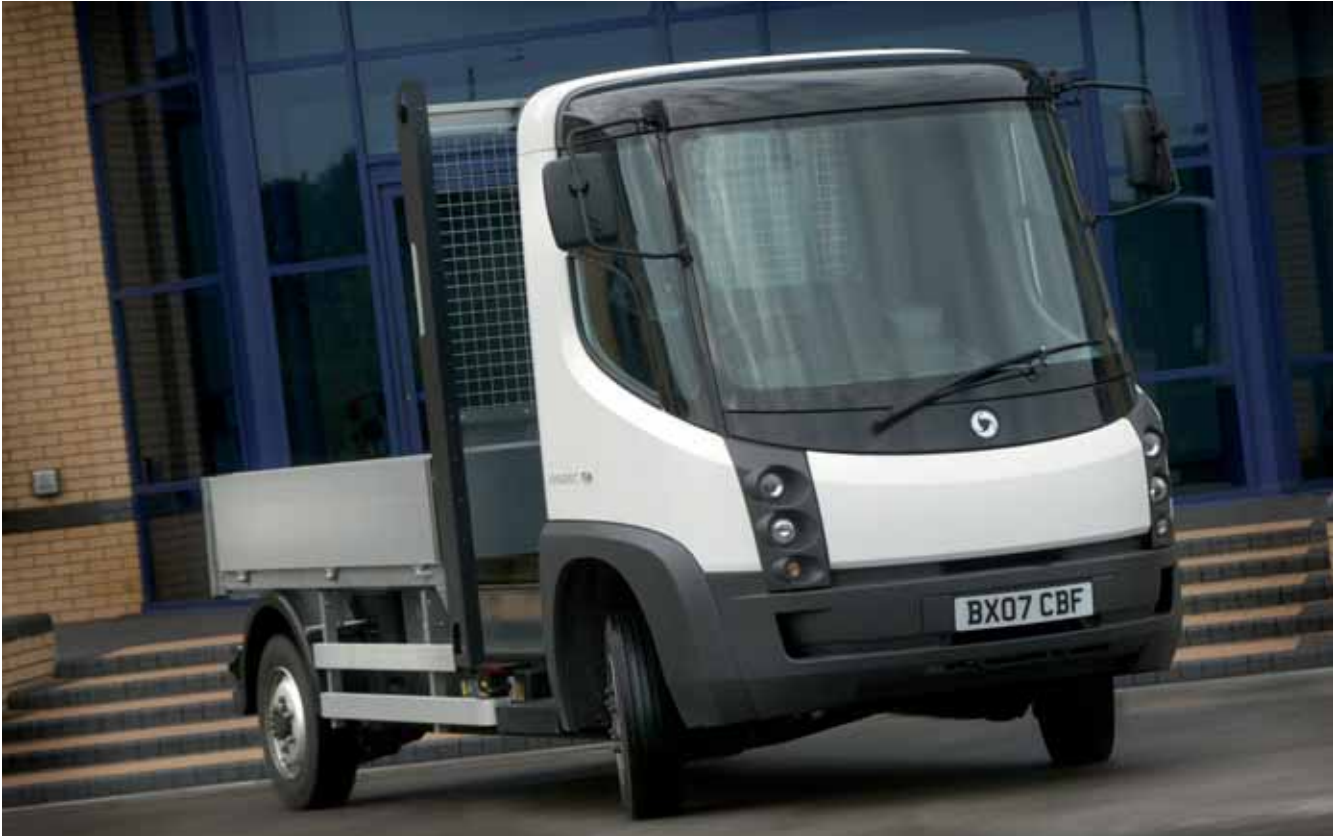
Modec's electric urban delivery van is powered by a ZyteK electric drivetrain
